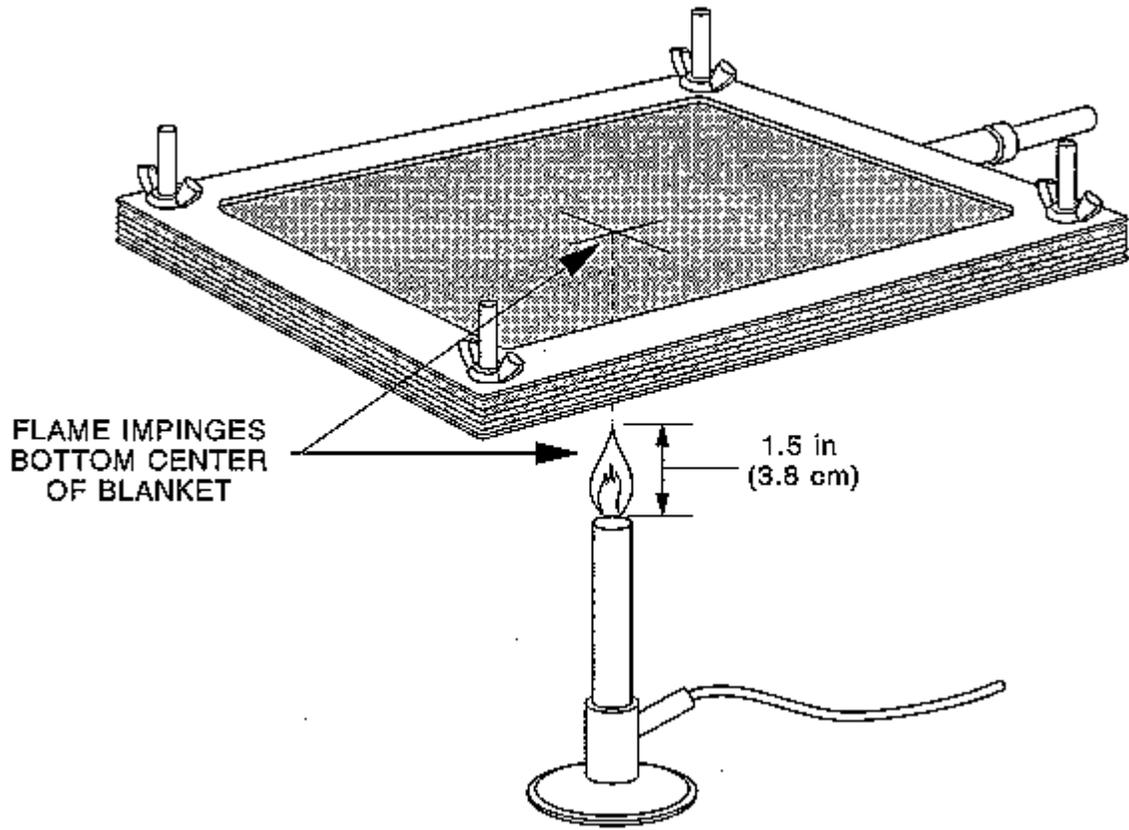
FIGURE B-6. HORIZONTAL TEST FIXTURE WITH 4-PLY BLANKET SAMPLE
