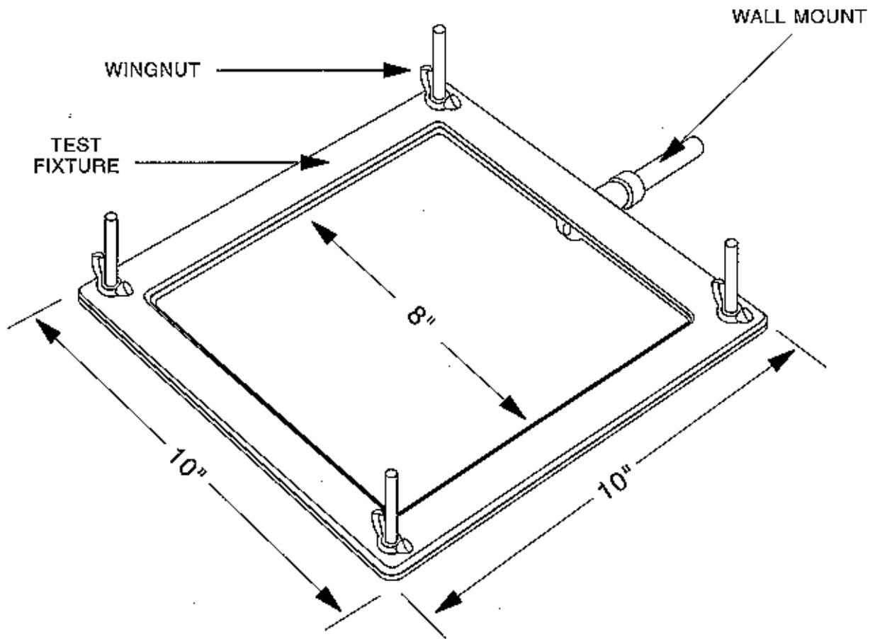
FIGURE B-4. HORIZONTAL TEST FIXTURE
